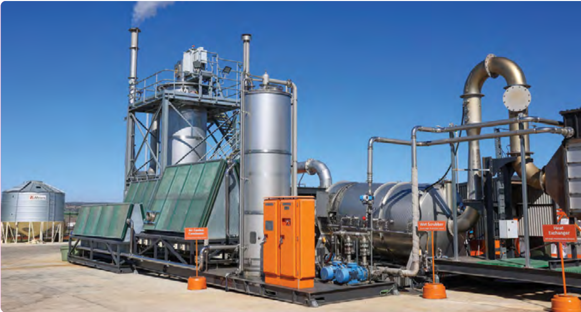
Pyrocal's Continuous Carbonisation Technology is being deployed in British Columbia at the Hartland Landfill to convert waste into valuable biochar.
